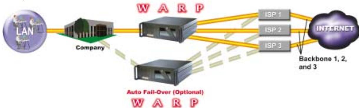
FatPipe WARP combines multiple routers into a single, high-speed Internet connection. In this diagram, two WARP units are used (called Dual WARP) for ultimate reliability.
