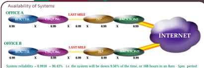
System reliability = 0.9910 = 90.43% i.e. the system will be down 9.56% of the time, or 168 hours in an 8am - 5pm period (220 days/yr). At \$10,000/hr, the cost to the company =  $168 \times $10,000 = $1,680,000/\text{year}$  for a two office connection
