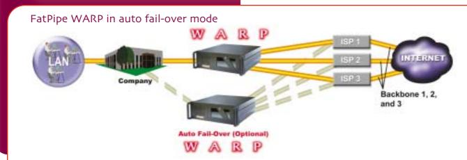
FatPipe WARP combines multiple routers into a single, high-speed Internet connection. In this diagram, two WARP units are used (called Dual WARP) for ultimate reliability.
