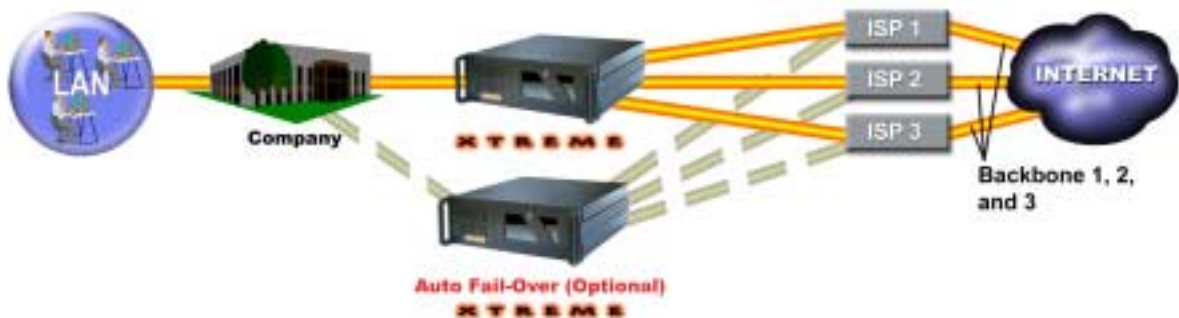
Figure 1: FatPipe Xtreme combines multiple routers into a single, high-speed Internet connection. In this diagram, two Xtreme units are used (called Dual Xtreme) for ultimate reliability.
