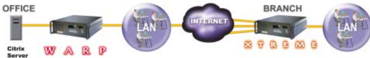
Figure 2: FatPipe Xtreme combines multiple routers into a single, high-speed Internet connection, while WARP provides high Wan availability for the server.
