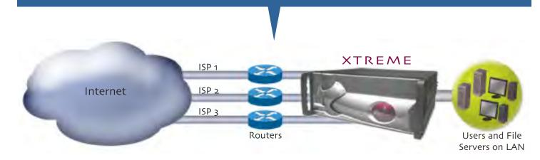
SUPERSTREAM has similar features and benefits as the FatPipe XTREME product, but in a compact 2 Mbps size to meet the needs of smaller companies and branch offices. Use SUPERSTREAM to aggregate two connections of any type of media (T1, DSL, Cable , Wireless, and/or ISDN) for increased WAN speed and reliability. Two additional WAN ports canbe enabled for up to four connections.
